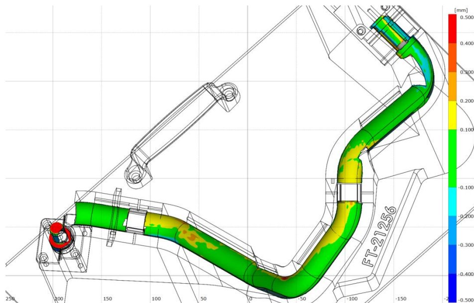
Figure 7. Deviation field of digitized surface in reference to CAD model of attribute check fixture.
